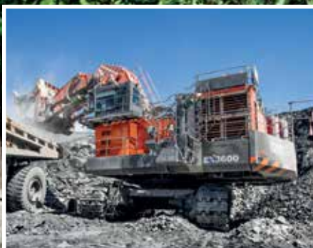
EX ultra-large excavators
